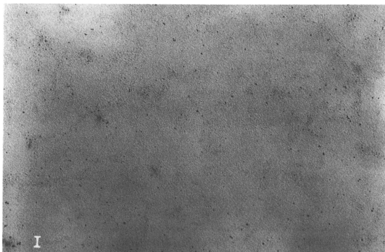
Figure 8. TEM picture showing catalyst particles in poly(3-chloro-2-hydroxypropyl-2-methacryloxyethyl-dimethyl ammonium chloride). Polymer : Pt = 25 : 1 (Mass) (Bar = 16 nm).
