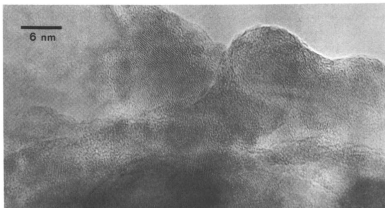
Figure 3. High-Resolution TEM of GaP Nanocrystals. The bar in the figure indicates a scale of 6 nm.
